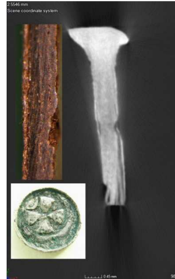
Fig. 2. From the left hand side: real photo and cross-section microscopic photo of silver medieval coins with zinc-copper core covered by silvering, X-ray CT grey-scale image with differing colour areas. The X-ray CT method can be use to detect coins with a core, mint forgeries.
