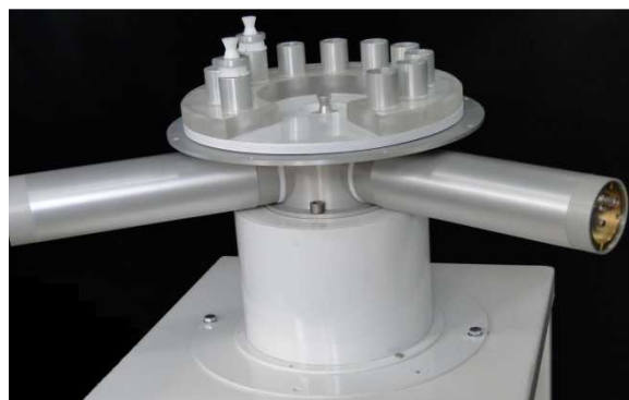
Fig. 2. Triple-to-double coincidence ratio system with additional gamma detector.
