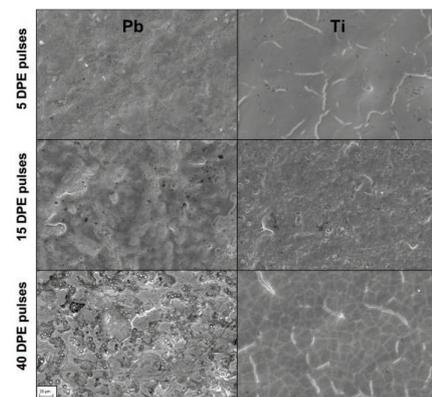
Fig. 2. Pb and Ti layers deposited on a Nb substrate using 5 plasma pulses with 5 J/cm<sup>2</sup> energy density, 15 plasma pulses with 5 J/cm<sup>2</sup>, and 40 plasma pulses with energy density decreasing from 7 J/cm<sup>2</sup> to 1 J/cm<sup>2</sup>.
