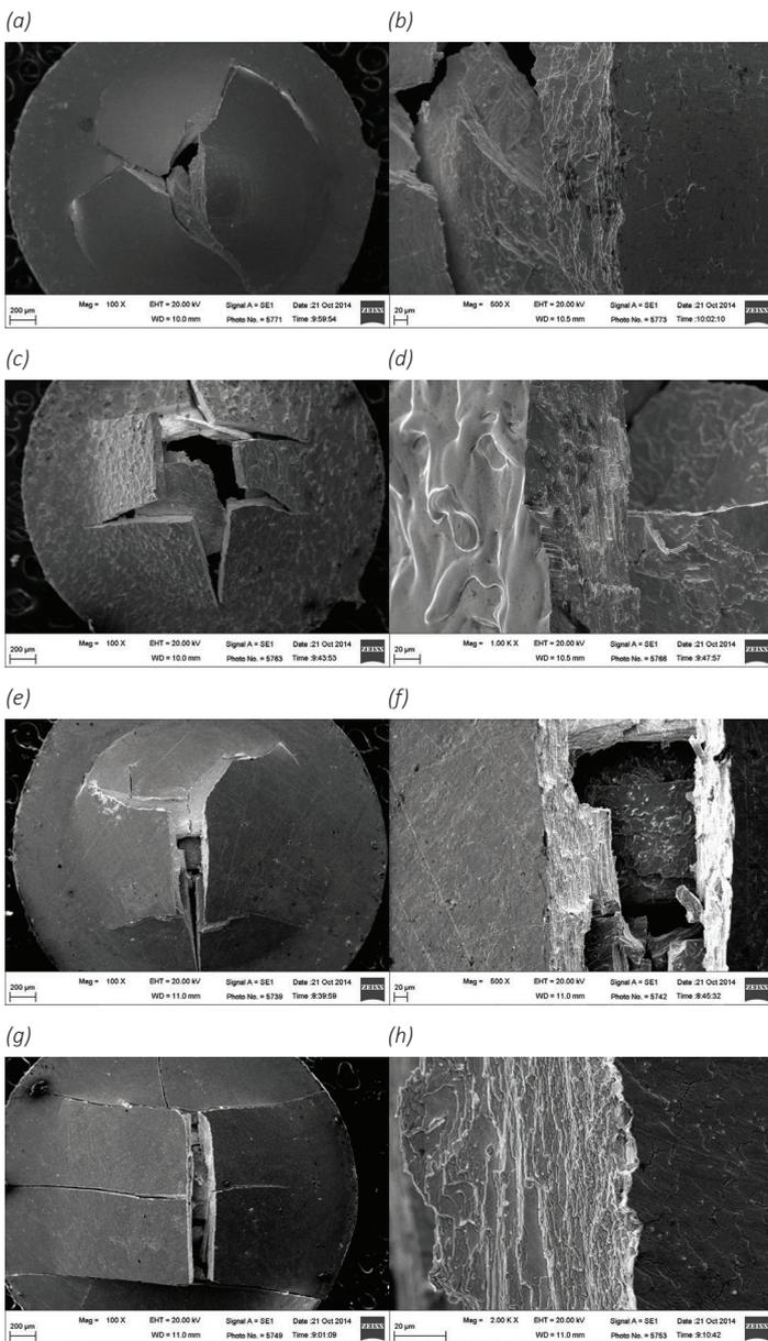
Fig.3. Fracture surfaces – SEM-photos; a, b/ initial state, c, d/ after plasma action, e, f/ after Ar ion irradiation, g, h/ after plasma action and Ar ion irradiation.
