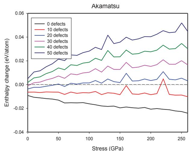
Fig.1. Variation of mean enthalpy per atom in MgO structure containing point defects as a function of the number of defects and stress level. Positive values mean that point defects are less energetically favourable than dislocations.
