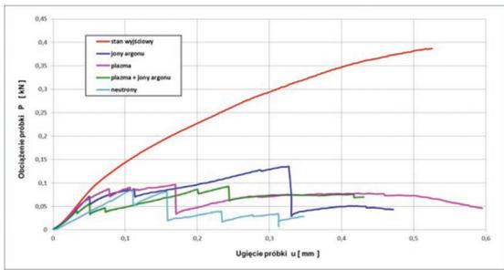
Fig.2. The force – deflection curves for different material states.
