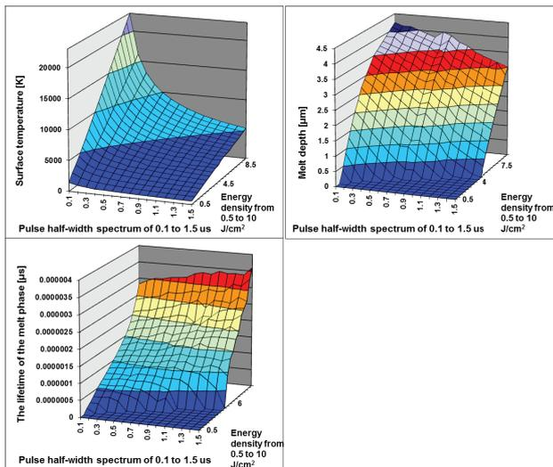
Fig. 1. Surface temperature, melt depth, lifetime of the melt phase as a functions of the pulse energy density and the pulse half-width, the pulse half-width spectrum from 0.1 to 1.5 ms and the energy density from 0.5 to 10 J/cm<sup>2</sup>.
