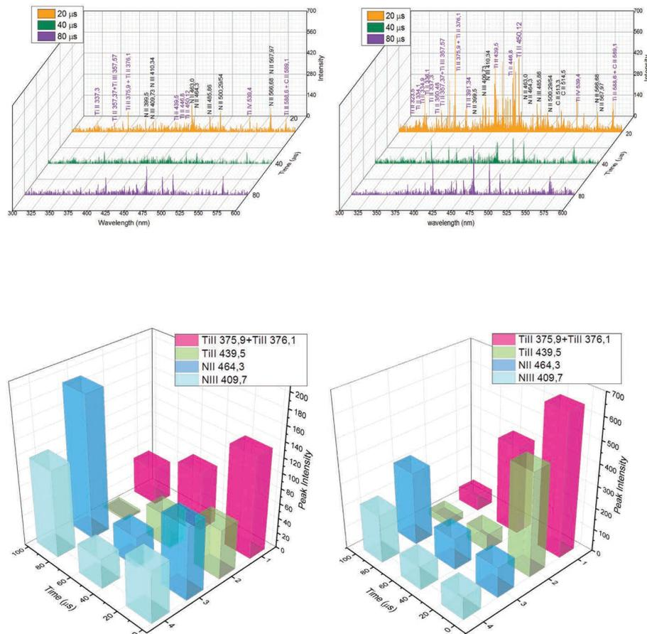
Fig. 1. Time resolved distribution of pulsed plasma for a 3 kV discharge (left graph) and for a 4 kV discharge (right graph). Time resolved distribution of chosen spectral lines (bottom).
